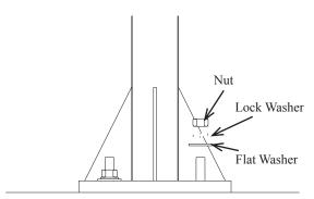
Figure 8 Securing the Pole to the Pad
